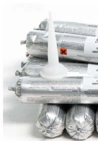
STARMASTIC P95 Mean elastic module one-component polyurethane sealant for flooring joints or special seals. This sealant bonds directly to concrete, marble, stone, steel, aluminium, glass, resin, wood and plastic. It can be overpainted with elastomers and has excellent elasticity and resistance to chemical agents and water.
